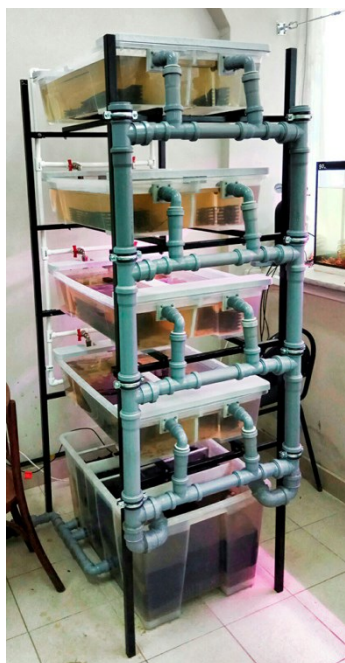
Fig. 1. A multi-tier recirculating water supply facility used to rear juvenile Australian red-clawed crayfish ( Cherax quadricarinatus ).
